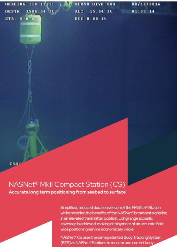
movement, thereby maintaining high accuracy positioning even in areas of strong seabed current.
