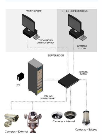
The system design allows for flexible configuration of operator stations together with a wide choice of camera viewing solutions with specific camera designs to suit all above-deck, below-deck and subsea monitoring applications. The system components can take full advantage of the latest IP network and Power-over-Ethernet (PoE) cabling infrastructure to simplify installation requirements, increase flexibility and significantly reduce vessel installation costs.
